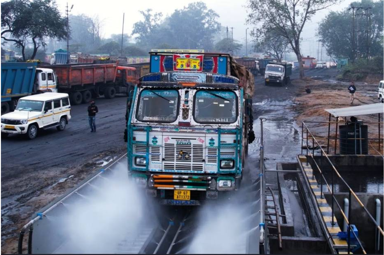
Wheel washing facility at Mine Barrier
