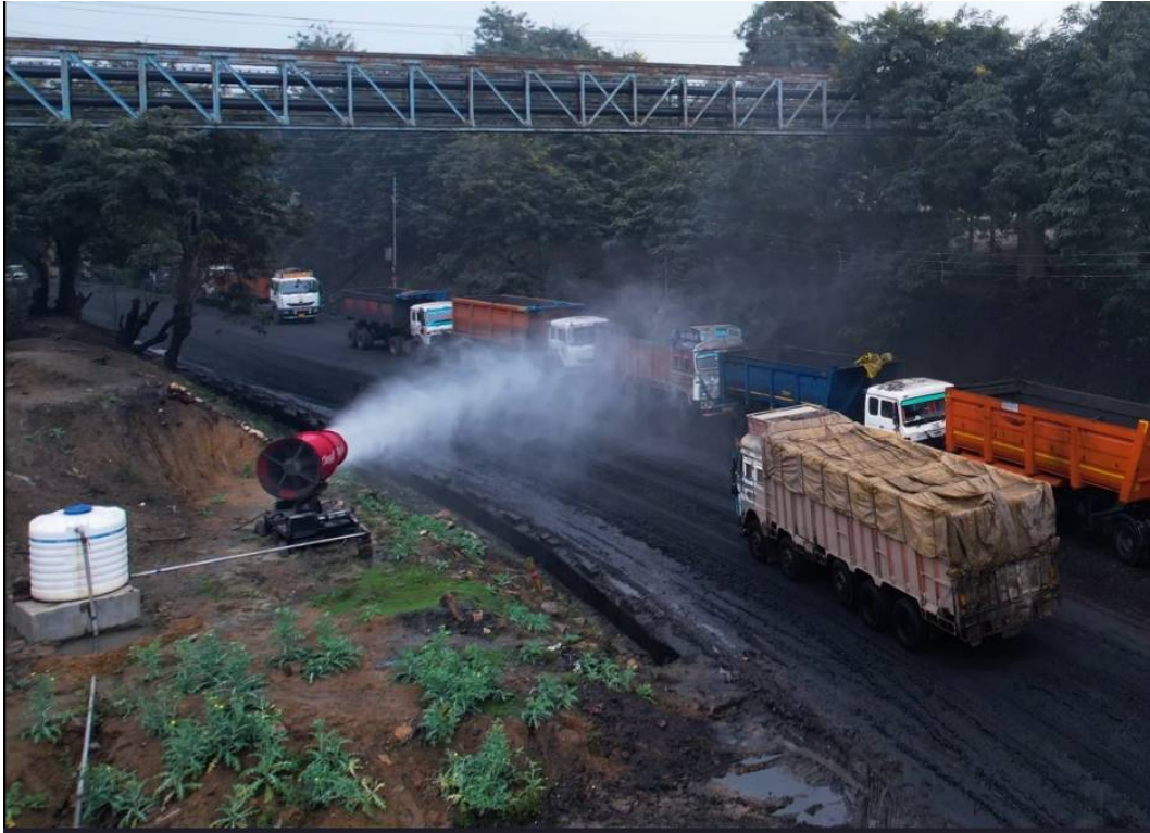
Fixed Fog Canon at Mine Barrier
